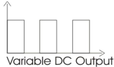
Chopper can increase or decrease the dc voltage level at its opposite side. So, chopper serves the same purpose in [DC circuit](#) transfers in case of ac circuit. So it is also known as DC transformer.
