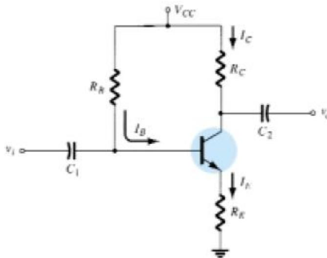
Fig.10: BJT bias circuit with emitter resistor.
