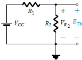
Fig.19: Determining  $E_{Th}$
