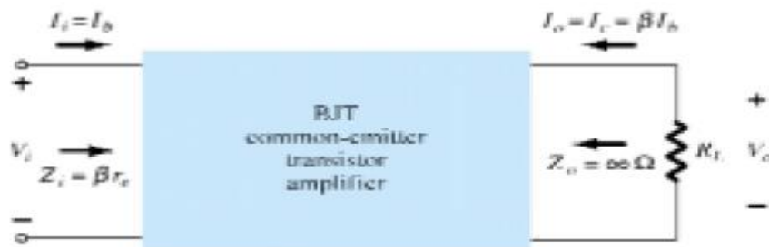
Fig.14: Determining the voltage and current gain for the common-emitter transistor amplifier.
