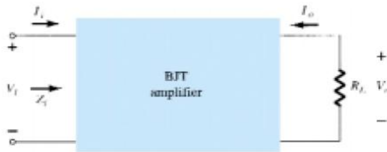
Fig.9: Determining the loaded current gain.
