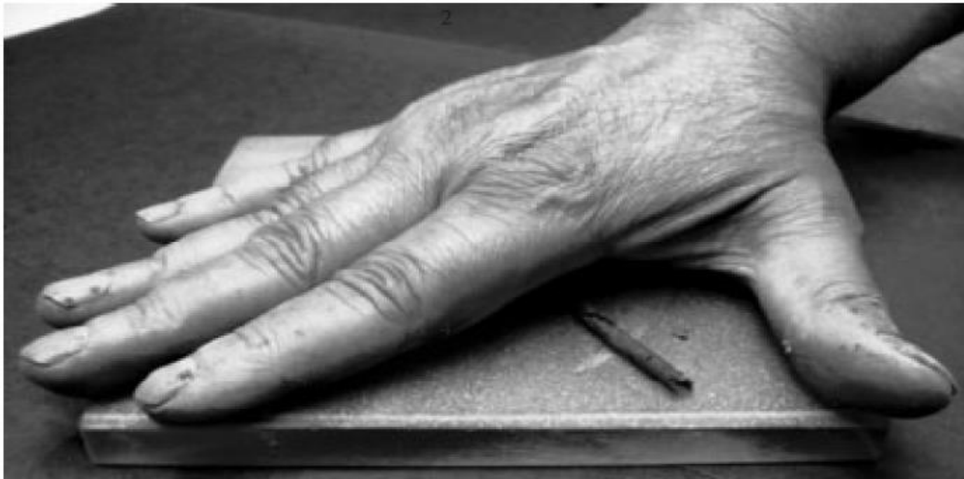
Figure 4.7 Rolling of soil mass on ground glass plate to determine plastic limit (Courtesy of Braja M. Das, Henderson, Nevada)
