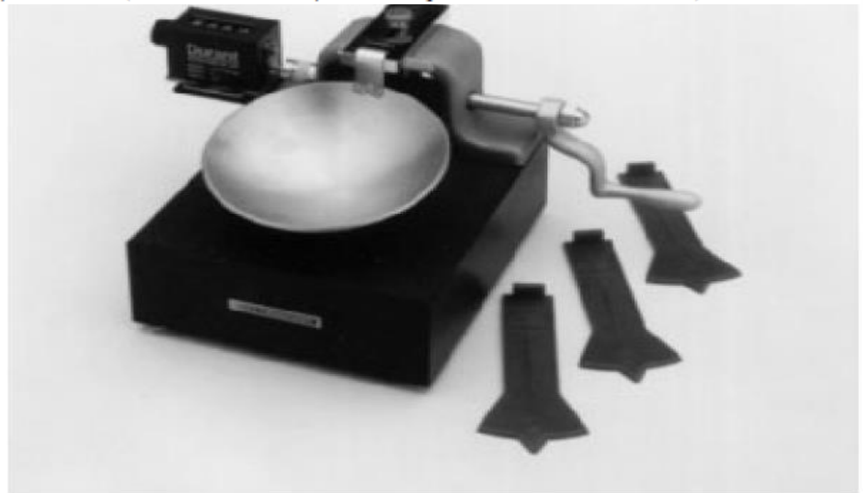
Figure 4.3 Liquid limit test device and grooving tools (Courtesy of ELE International)
