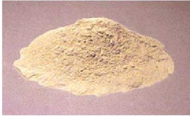
Fig. 3-2. Fly ash, a powder resembling cement, has been used in concrete since the 1930s. (69799)
