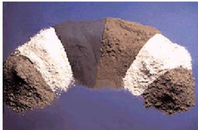
Fig. 3-1. Supplementary cementing materials. From left to right, fly ash (Class C), metakaolin (calcined clay), silica fume, fly ash (Class F), slag, and calcined shale. (69794)
