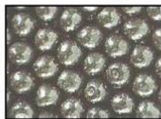
Lead Shot Aggregate Used for Radiation Shielding.
