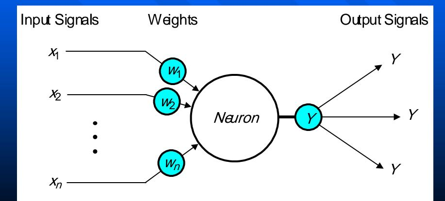
The neuron computes the sum of weighted input signals and compares the result with a threshold value, θ. If the net input is less than the threshold, the neuron output is -1. But if the net input is greater than or equal to the threshold, the neuron becomes activated and its output attains a value +1.
