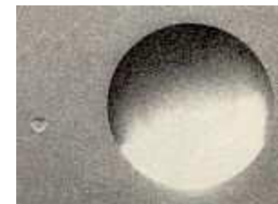
Brinell hardness impression
