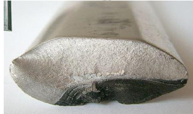
Fatigue failure in an Aluminium bicycle crank. Dark area of striations: slow crack growth. Bright granular area: sudden fracture
