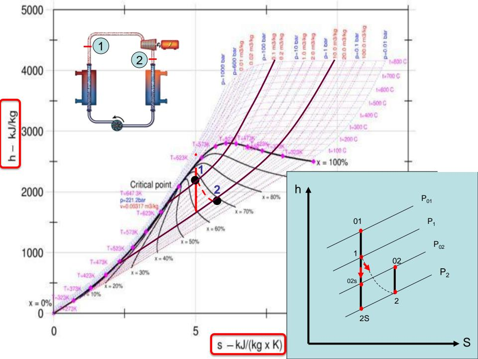
the static condition of the fluid at inlet is determined by state 1 with state ( <u>01 as the corresponding stagnation state</u>). the final static properties are determined by the state 2 with ( <u>02 as the corresponding stagnation state</u>). If the process were reversible, the fluid static state would be <u>2s</u> and the stagnation state be
