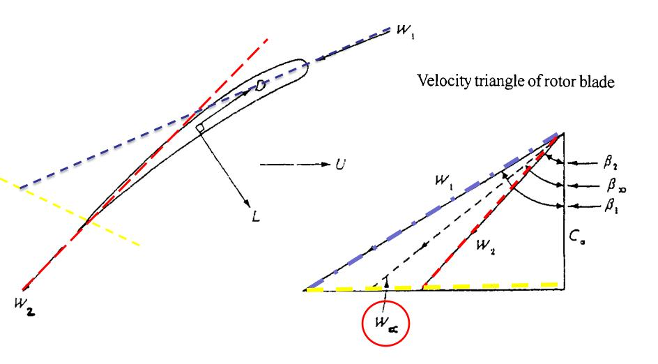
Consider a rotor blade shown in the figure with : W1,W2 = relative velocity vectors at inlet & outlet , W $\alpha$  = resultant velocity  $\beta_1$ = relative inlet air angle ,  $\beta_2$ = relative outlet air angle ,  $\beta\alpha$  = mean flow angle =45°
