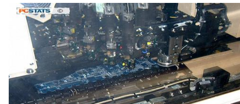
Each of the 16 or so heads places a different component in as little as 1/8 of a second (flash frozen in this picture)
