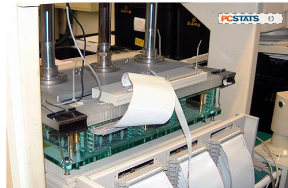
The rack is lowered, making contact with test points on the board
