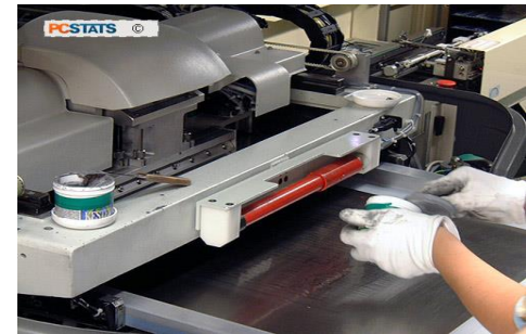
Mixing and applying the solder paste to the nickel screen
