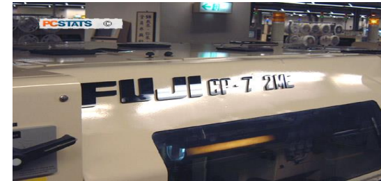
The FUJI pick and place SMT machines mount components on each motherboard
