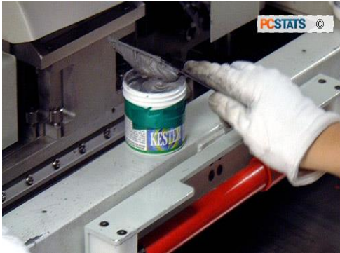
The solder paste: particles of solder suspended in flux
