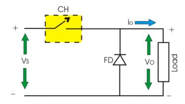
When CH is turned ON,  $V_s$  directly appears across the load as shown in figure.
