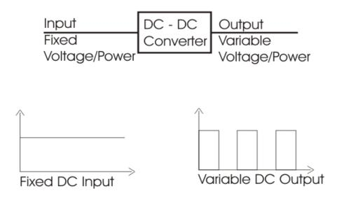
Chopper can increase or decrease the dc voltage level at its opposite side. So, chopper serves the same purpose in <u>DC circuit</u> transfers in case of ac circuit. So it is also known as DC transformer.
