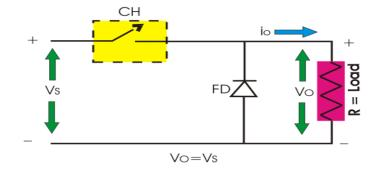
Average output voltage  $V_O = \frac{1}{T} \int_0^{T_{ON}} V_s dt = \frac{V_s T_{ON}}{T} = DV_s$
