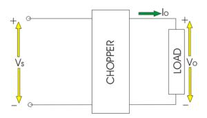
If output voltage ( $V_0$ ) and output current ( $I_0$ ) follows the direction as marked in figures then the chopper operation will be restricted in the first quadrant of  $V_0 - I_0$  plane. This type of operation is also known as forward motoring.
