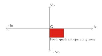
N ow we can proceed to detailed analysis of different types of chopper. Some choppers operate in a single quadrant only, which are called single quadrant chopper. Some choppers operate in two quadrant also which are known as two quadrant chopper. It is also possible that a chopper operates in all the quadrants, which are known as 4-quadrant chopper.
