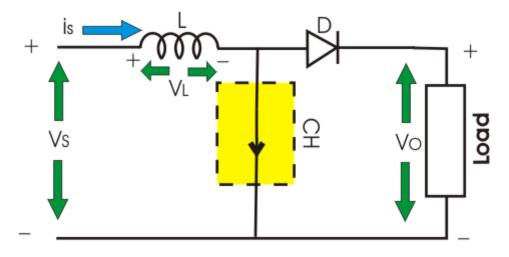
Where  $\Delta I$  is the peak to peak inductor current. When CH is OFF inductor L discharges through the load. So, we will get summation of both source voltage V<sub>s</sub> and inductor Voltage V<sub>L</sub> as output voltage, i.e.
