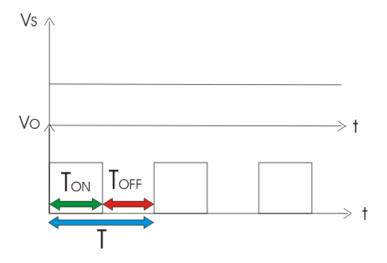
$T_{ON} \rightarrow It$  is the interval in which chopper is in ON state.  $T_{OFF} \rightarrow It$  is the interval in which chopper is in OFF state.  $V_S \rightarrow Source$  or input voltage.  $V_O \rightarrow Output$  or load voltage.  $T \rightarrow Chopping period = T_{ON} + T_{OFF}$
