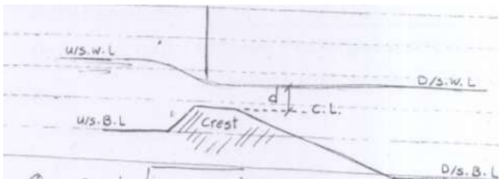
(Fully gate opening, floor with crest)
