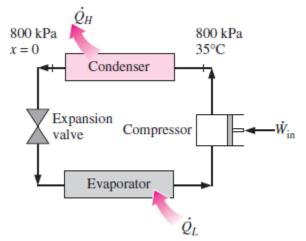
6-55 Refrigerant-134a enters the evaporator coils placed at the back of the freezer section of a household refrigerator at 120 kPa with a quality of 20 percent and leaves at 120 kPa and \_20°C. If the compressor consumes 450 W of power and the COP the refrigerator is 1.2, determine (*a*) the mass flow rate of the refrigerant and (*b*) the rate of heat rejected to the kitchen air.
