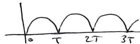
$$\begin{aligned} \mathcal{L}\{f(t)\} &= \int_0^\infty f(t) e^{-st} dt = \int_0^T f(t) e^{-st} dt + \int_T^{2T} f(t) e^{-st} dt \\ &\quad + \int_{2T}^{3T} f(t) e^{-st} dt + \dots \end{aligned}$$
