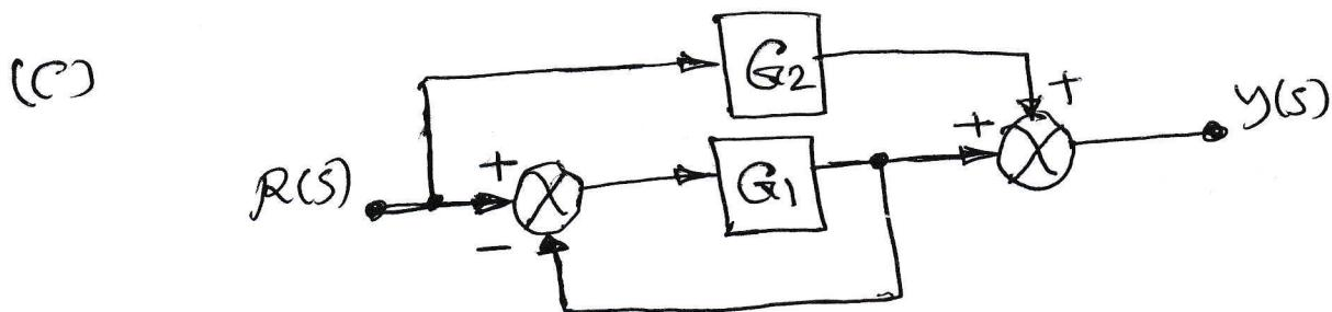
Q2 Find the transfer function for the block diagrams using Mason's rule.
