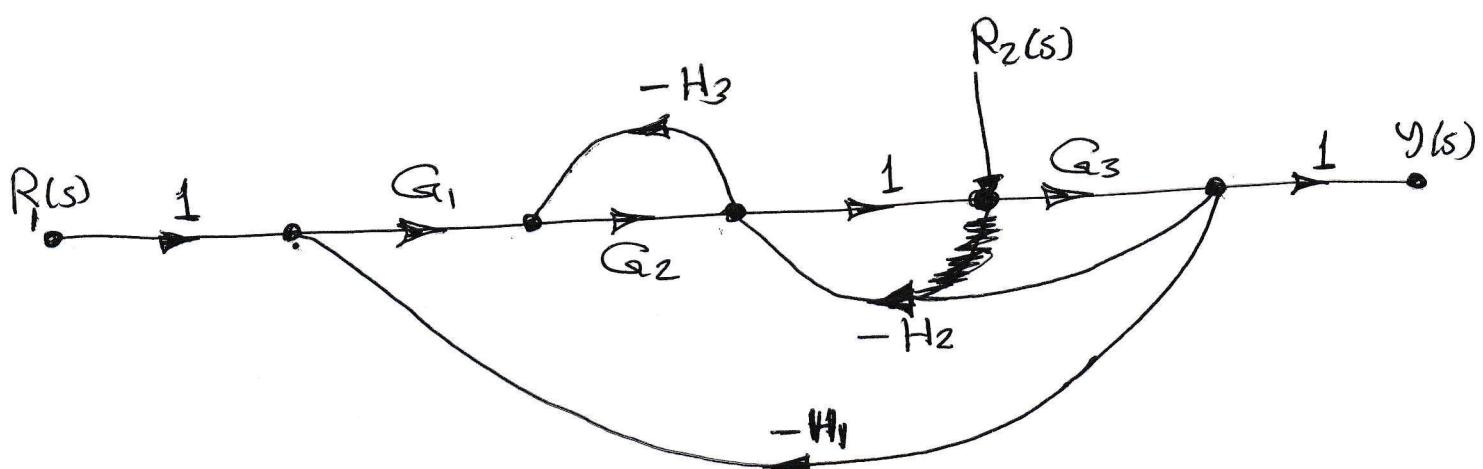
① for Transfer function  $\frac{Y(s)}{R_1(s)}$ ,  $R_2(s) = 0$
