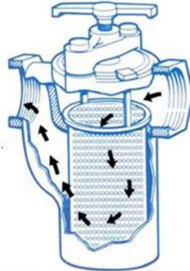
Flow Path Through a Basket Strainer
