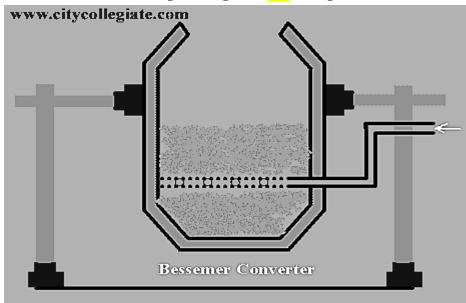
The copper so obtained is called "Blister copper" because, as it solidifies,  $SO_2$  hidden in it escapes out producing blister on its surface.
