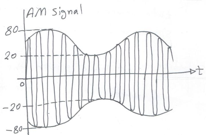
Ex. A carrier wave is represented by expression  $V_c(t) = 10 \sin \omega t$ . Draw the waveform of an AM wave for  $m_a = 0.5$ , and 1 Hz modulating signal.
