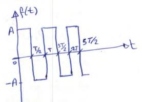
Q/Obtain the trigonometric Forier series for the waveform
