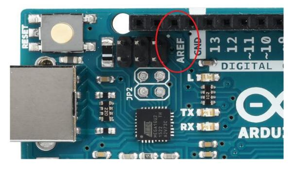
Alternatively, you can connect the external reference voltage to the AREF pin through a 5K resistor, allowing you to switch between external and internal reference voltages.
