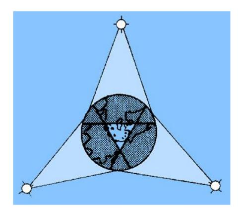
Figure 1-9. - Worldwide synchronous satellite system viewed from above the North Pole
