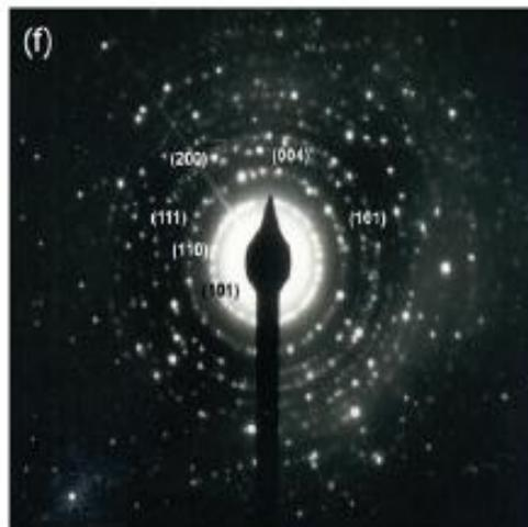
(a and b) TEM photographs of  $n\text{-TiO}_2$  synthesized respectively using *Lactobacillus* sp. and yeast. The inset in A and B are the deposition of  $n\text{-TiO}_2$ . (c and d) Particle size distribution (%). (e and f) SAED patterns of  $n\text{-TiO}_2$  (upper: *Lactobacillus* assisted and lower: yeast assisted synthesis).
