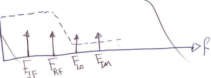
Second case :  $RF > LO$ , hence,  $F_{IM} = 2F_{IF}$  below RF, in this case,  $F_{IM}$  is inside the LRF, therefore, a BPF (sharp) must be used to attenuate the image frequency.
