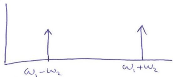
Generally speaking, two inputs (RF & Image) will mix to the same output (IF) frequency
