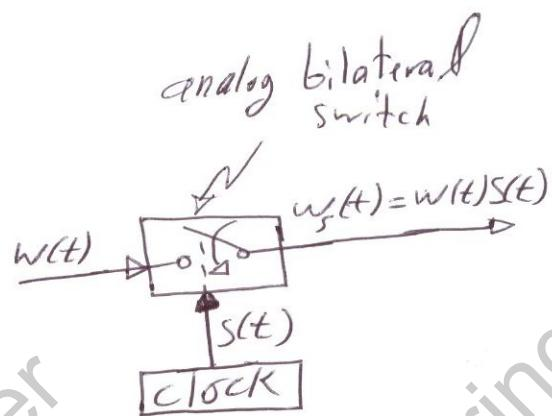
Ex. For an input waveform of rectangular spectrum of bandwidth  $B$  Hz, draw the natural sampled version of this input signal and calculate the PAM bandwidth if you know that the sampling frequency  $f_s = 4B$  Hz and the duty cycle of the switching waveform is  $d = \tau/T_s = \frac{1}{3}$ .
