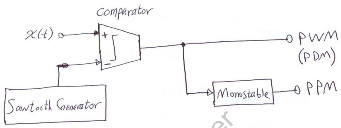
\* The output of the comparator is zero except when the message waveform  $x(t)$  is the sawtooth waveform.
