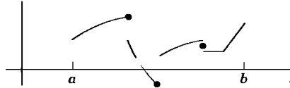
Fig. 114. Example of a piecewise continuous function f(t) . (The dots mark the function values at the jumps.)
