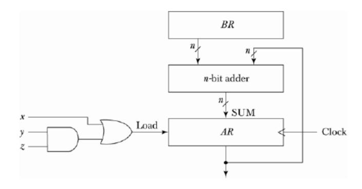
4-9. Show the hardware that implements the following statement. Include the logic gates for the control function and a block diagram for the binary counter with a count enable input.
