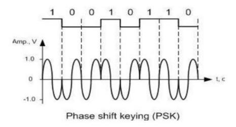
PSK - phase of carrier signal is varied to represent binary 1 or 0
