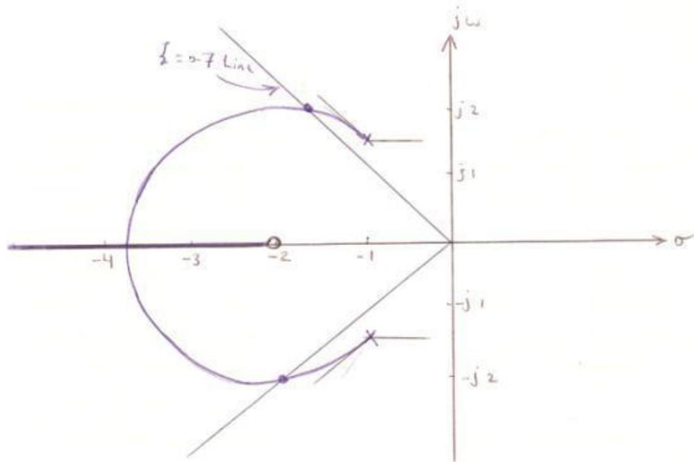
The value of the gain  $K$  at any point on the root locus can be found by applying the magnitude condition.
