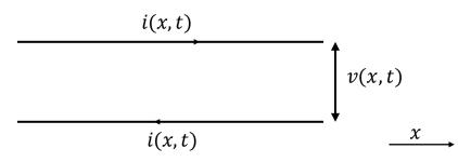
It is possible to show, using basic laws of electrical circuit theory, that the electrical current i(x, t) satisfies the PDE:
