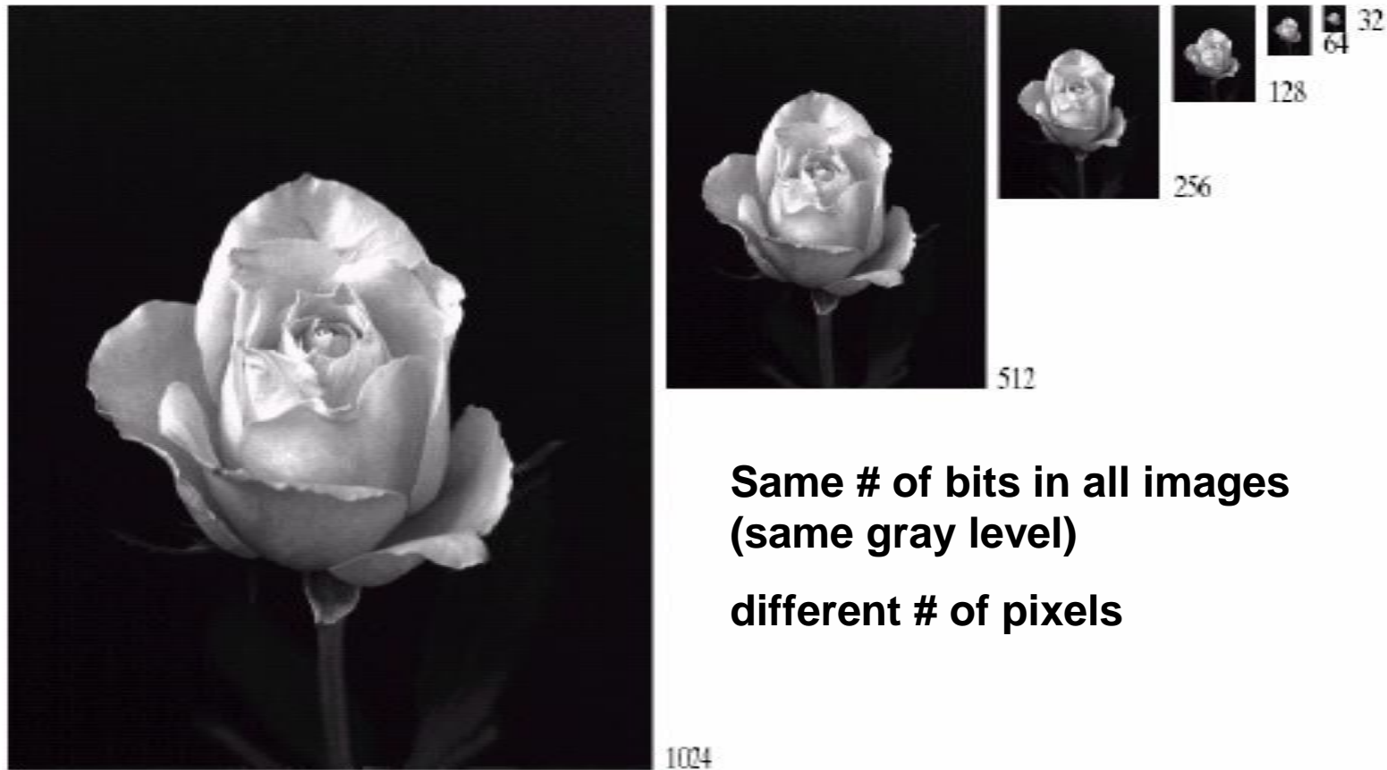
FIGURE 2.19 A 1024 \times 1024 , 8-bit image subsampled down to size 32 \times 32 pixels. The number of allowable gray levels was kept at 256.
