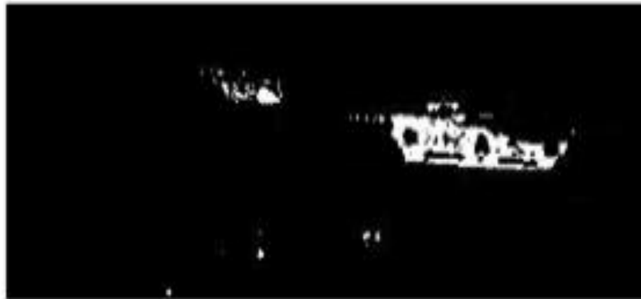
(c) Subtracting image (b) from (a). Only moving objects appear in the resulting image
