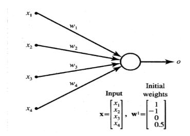
Step 1 Input  $x_1$  applied to the network results in activation  $net^1$  as below:
