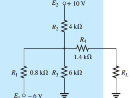
$$R_{Th} = R_4 + R_1 || R_2 || R_3$$
