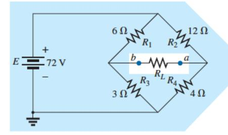
$R_{Th} = R_{a-b} = R_1 || R_3 + R_2 || R_4$  $= 6 \Omega || 3 \Omega + 4 \Omega || 12 \Omega$  $= 2 \Omega + 3 \Omega = 5 \Omega$
