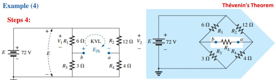
$$V_{1} = \frac{R_{1}E}{R_{1} + R_{3}} = \frac{(6 \ \Omega)(72 \ V)}{6 \ \Omega + 3 \ \Omega} = \frac{432 \ V}{9} = 48 \ V$$
