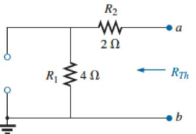
$R_{Th} = R_1 + R_2 = 4 \ \Omega + 2 \ \Omega = 6 \ \Omega$
