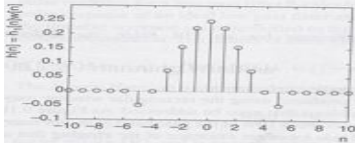
(c)(i) Impulse Response for Non-Ideal Low Pass Filter
