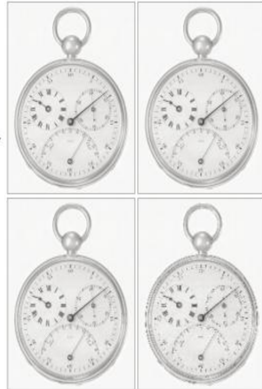
FIGURE 2.20 Typical effects of reducing spatial resolution. Images shown at: (a) 1250 dpi, (b) 300 dpi, (c) 150 dpi, and (d) 72 dpi. The thin black borders were added for clarity. They are not part of the data.
