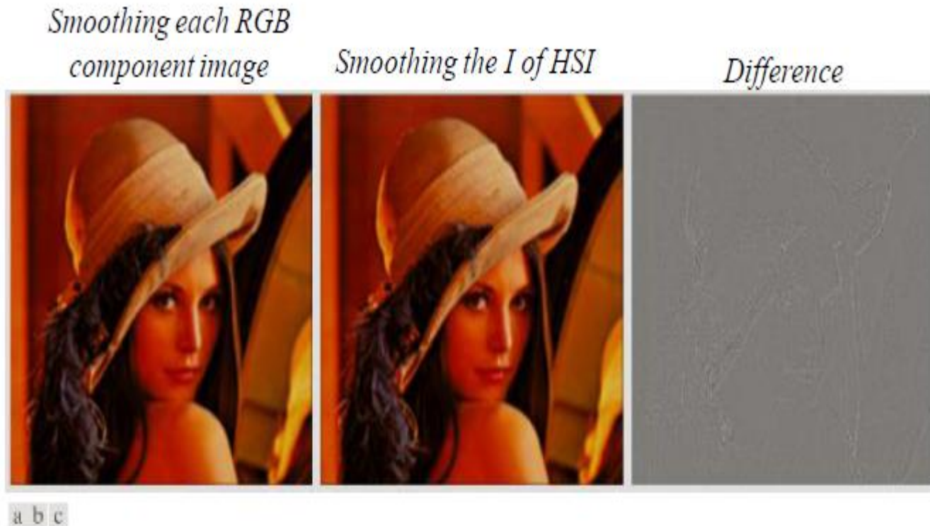
FIGURE 6.40 Image smoothing with a 5 \times 5 averaging mask. (a) Result of processing each RGB component image. (b) Result of processing the intensity component of the HSI image and converting to RGB. (c) Difference between the two results.
