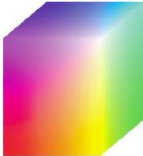
FIGURE 6.8 RGB 24-bit color cube.
